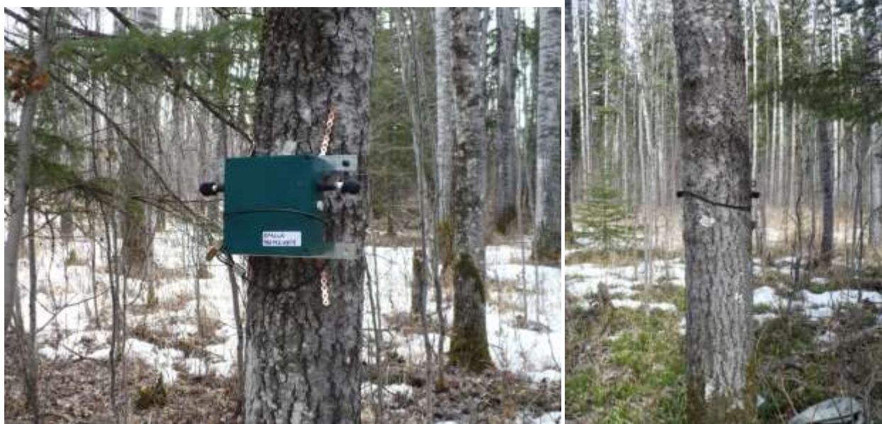
Figure 1. ARU placement on tree. Maximum width of tree. Microphones still are wider than the trunk, thus avoiding sound shadow from the tree.
