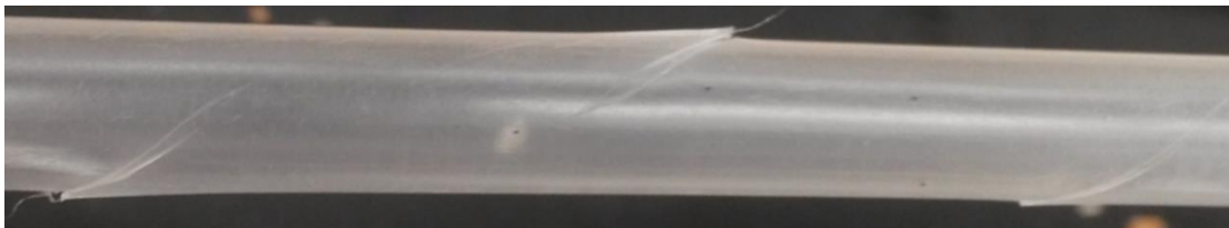
Figure 18. Straws are cut halfway through at a consistent angle from both sides to allow samples to dry and to avoid mold/rot
