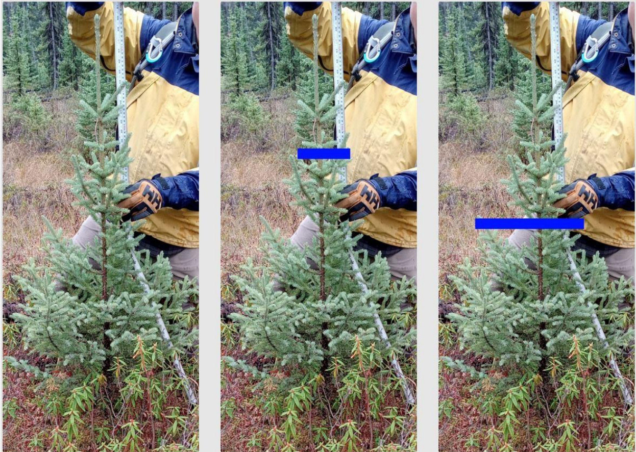
Figure 20. Example of pixel size at 15 cm (middle) and 30 cm (right) projected vertically at the black spruce sapling. The mass of vegetation large enough to be displayed at the minimum pixel size (15 cm, 30 cm respectively), indicated by the blue marker line, is offset from the measured height by approximately 30 cm (for GSD 15cm) and by 45 cm (for GSD 30 cm).
