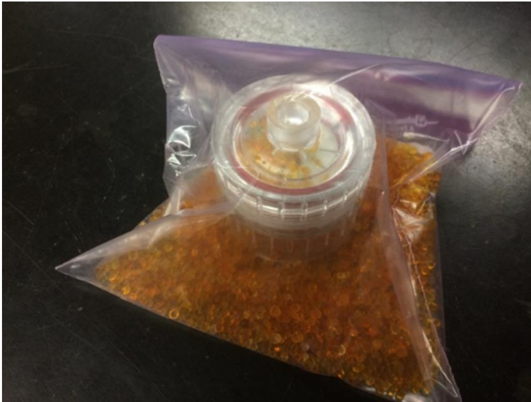
Figure 5. Ziploc bag with desiccant beads inside of the filter housing. Photo Credit: Jim Davies (InnoTech Alberta).
