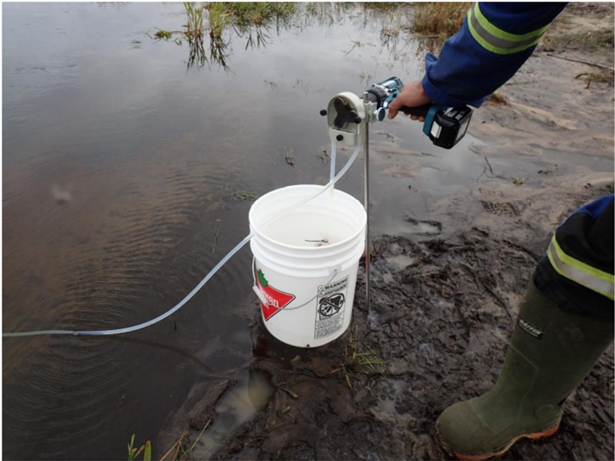
Figure 3. Set-up of filtration assembly and field-deployable peristaltic pump attached to metal spike for taking a sample. Photo Credit: Jim Davies (InnoTech Alberta)
