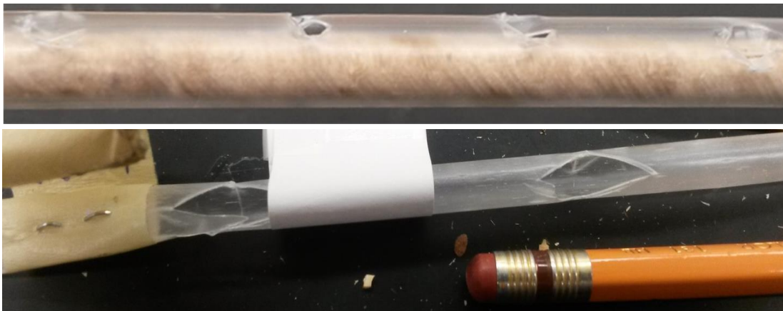
Figure 19. The two images above are examples of unacceptable punctured straws. The top straw has punctures that are too small and are pointing inwards potentially damaging the core. The bottom straw has punctures that are large enough for pieces of the core to break and escape the straw.
