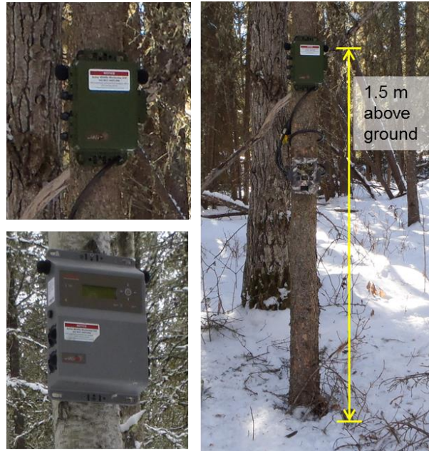
Figure 7. ARU placement on a tree. Microphones are wider than the trunk, thus ensuring that sound is not blocked by the tree.
