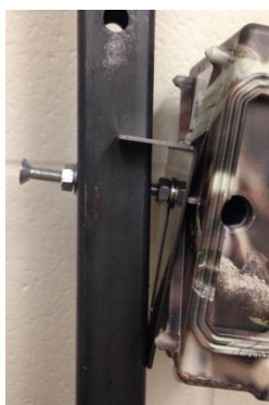
Figure 8. Custom A-bracket attached between the post and camera to adjust the tilt of the unit.
