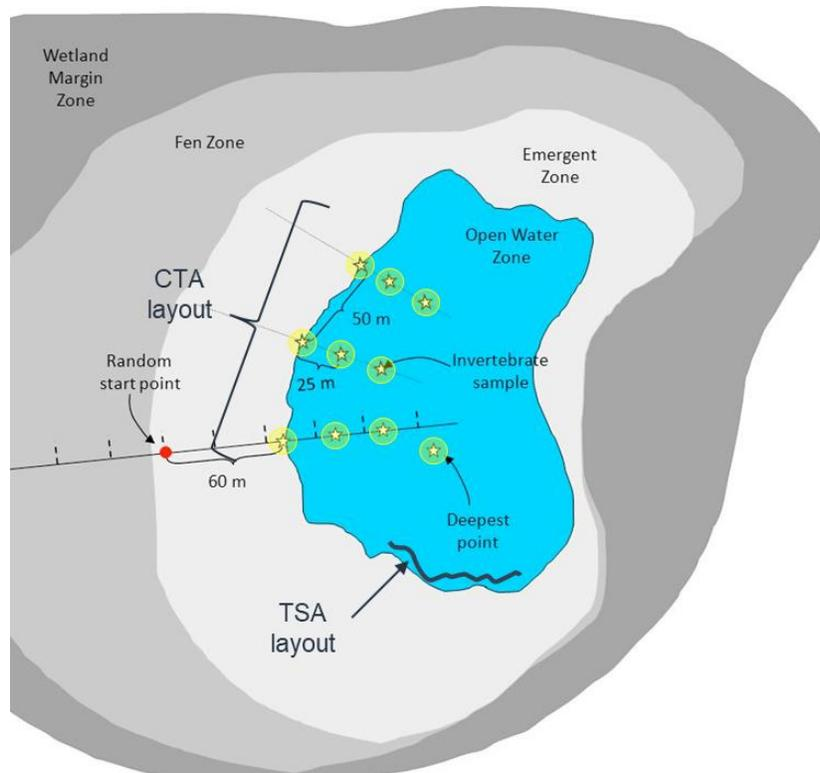
Figure 2 - Diagram of the CTA aquatic invertebrate sampling layout and the general placement of the TSA net sweep layout.
