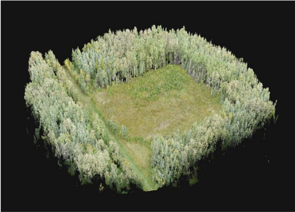
Figure 8. Three-dimensional view of the UAV photogrammetric point cloud for a reclaimed wellsite. Adapted from Hird and McDermid (2015).
