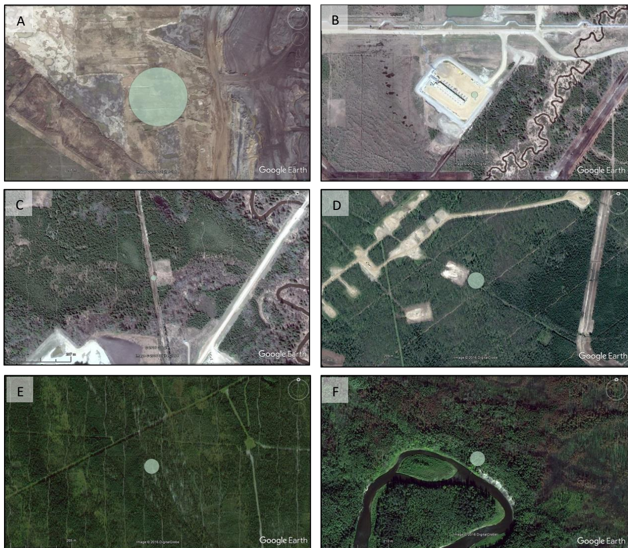
Figure 7.2. Examples of footprint types associated with provincial records of rare vascular plant populations in the oil sands area of Alberta. A) Population likely lost to conventional surface mining, B) Population likely lost to commercial in-situ, C) Developing in-situ likely impacting population, D) Developing in-situ adjacent to population, E) Exploratory seismic development adjacent to population, F) Undisturbed population. All maps created from Google Earth version 7.1.7.2026, imagery from DigitalGlobe 2016.
