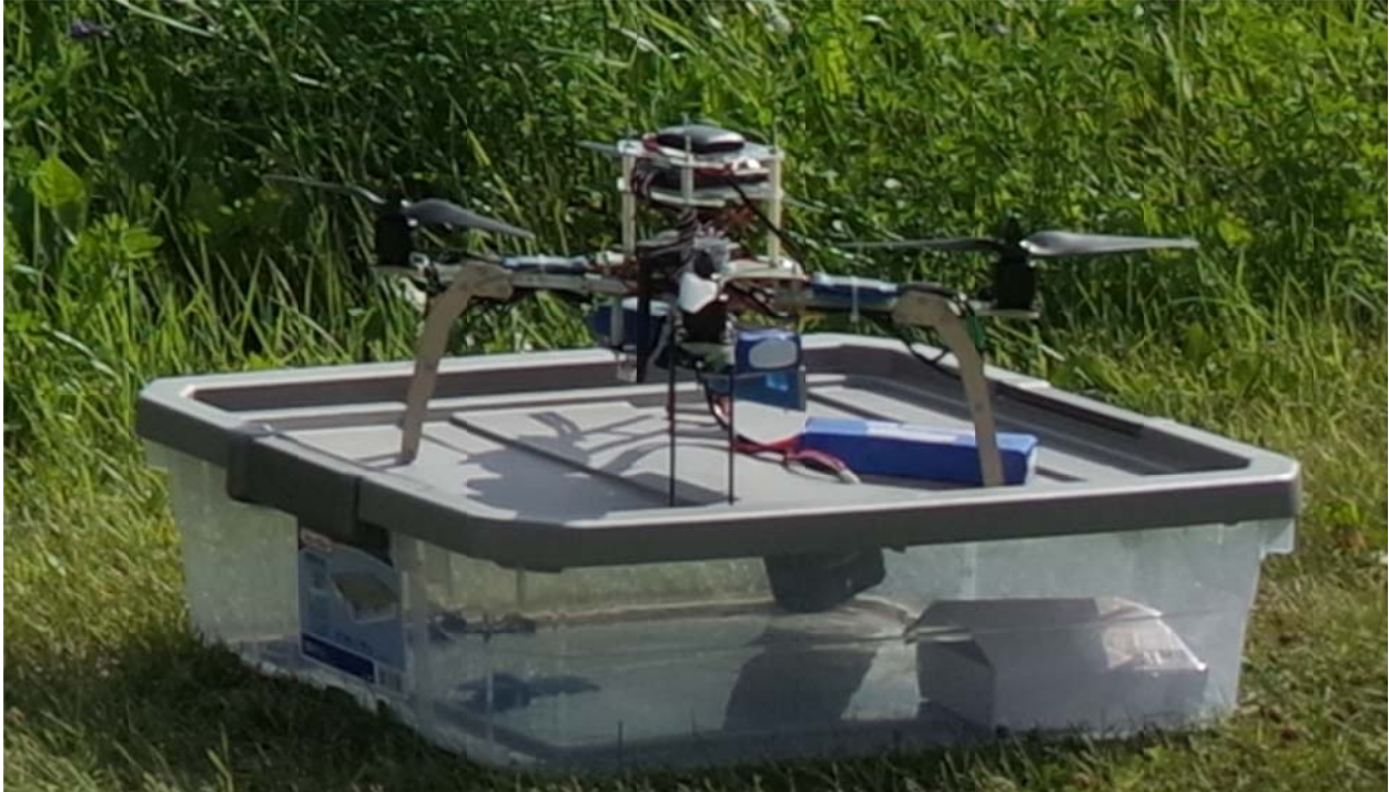
Figure 6. Photograph of prototype UAV in the field preparing to undergo a trial flight. The blue objects are the 5 Ah lithium-polymer batteries. The camera has been removed for arming.
