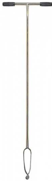
Fig.14. a) Dutch auger and b) Bucket auger
