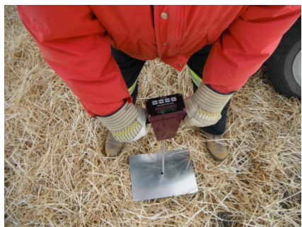
Fig. 13. Digital penetrometer (Spectrum Technologies FieldScout SC 900 Soil Compaction Meter).
