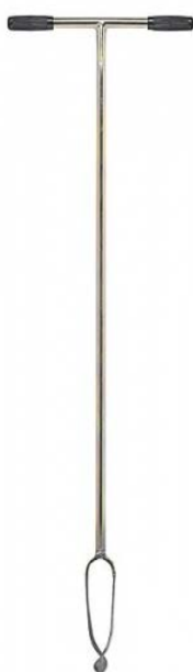
Fig.14. a) Dutch auger and b) Bucket auger
