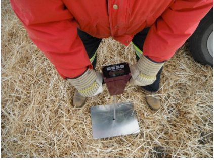
Fig. 9. Digital penetrometer (Spectrum Technologies FieldScout SC 900 Soil Compaction Meter).
