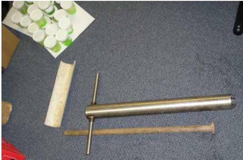
Figure 1: Picture of corer designed to collect soil cores for ABMP arthropod collection.
